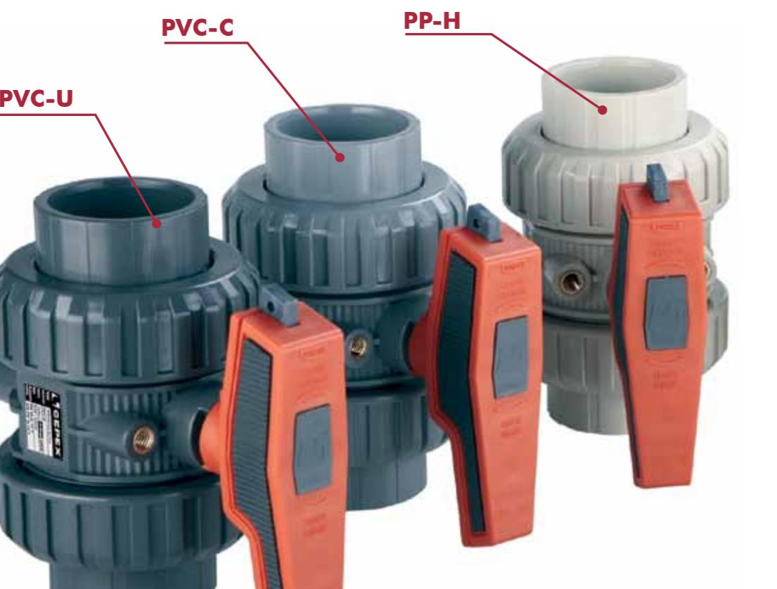
New range of ball valves in its [IND] Series, available in PVC-U, PVC-C, PP-H (handle in PP-GR + TPE, PTFE seats, food grade EPDM or FPM sealing). Sizes from D20 up to D110 (½" to 4"). The valve represents a major step forward both for its design and new features, offering the following characteristics:
