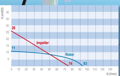
JP-360, 230 VAC, JP-PP(HC)41-1,000, test media water 20°C, pressure pipe 1", oval gear meter, measured values: ± 5%
