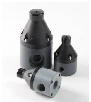
**Griffco G-Series** diaphragm pressure relief valves are designed to protect chemical feed systems from over pressure damage caused by defective equipment or a blockage in the chemical feed line. Robust construction ensures reliability in the rigorous service of municipal and industrial applications. Wetted materials include: **PVC, CPVC, PP, PVDF, PTFE, Halar, 316 SS, A20 and Hastalloy C**. Available sizes: 1/2" - 4".
