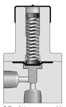
Griffco diaphragm pressure relief valves are designed to protect chemical feed systems from over pressure damage caused by defective equipment or a blockage in the chemical feed line. Robust construction ensures reliability in the rigorous service of municipal and industrial applications. Wetted materials include 316 SS, A 20 and Hast. C. Available sizes: 1/4", 3/8", 1/2", 3/4" and 1"
