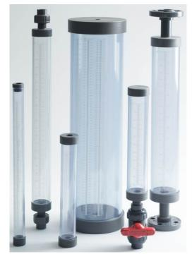
**Griffco** calibration cylinders are designed to enhance the performance of chemical feed systems by providing a verification of the flow rate of the chemical feed pump. Robust construction of clear PVC with an easy to read graduation in mL and gph. Available in three models: EZ-Clean, Vented, and Open Top; and in 15 sizes: 100 mL through 40,000 mL as detailed here.
