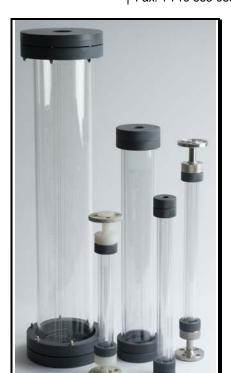
Griffco Borosilicate Glass Calibration Cylinders are designed to enhance the performance of chemical feed systems by providing a verification of the flow rate of the chemical feed pump. Constructed of borosilicate glass and a choice of 8 end cap materials, (PVC, CPVC, PP, PTFE, PVDF, 316SS, Alloy 20, and Hastelloy C) these cylinders are suitable for use with most chemicals. Available in 12 sizes; from 30mL to 20 L.
