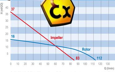
JP-480, 230 VAC, JP-SS 41-1000, test media water 20 °C, pressure pipe 1", oval gear meter, measured values: ± 5%
